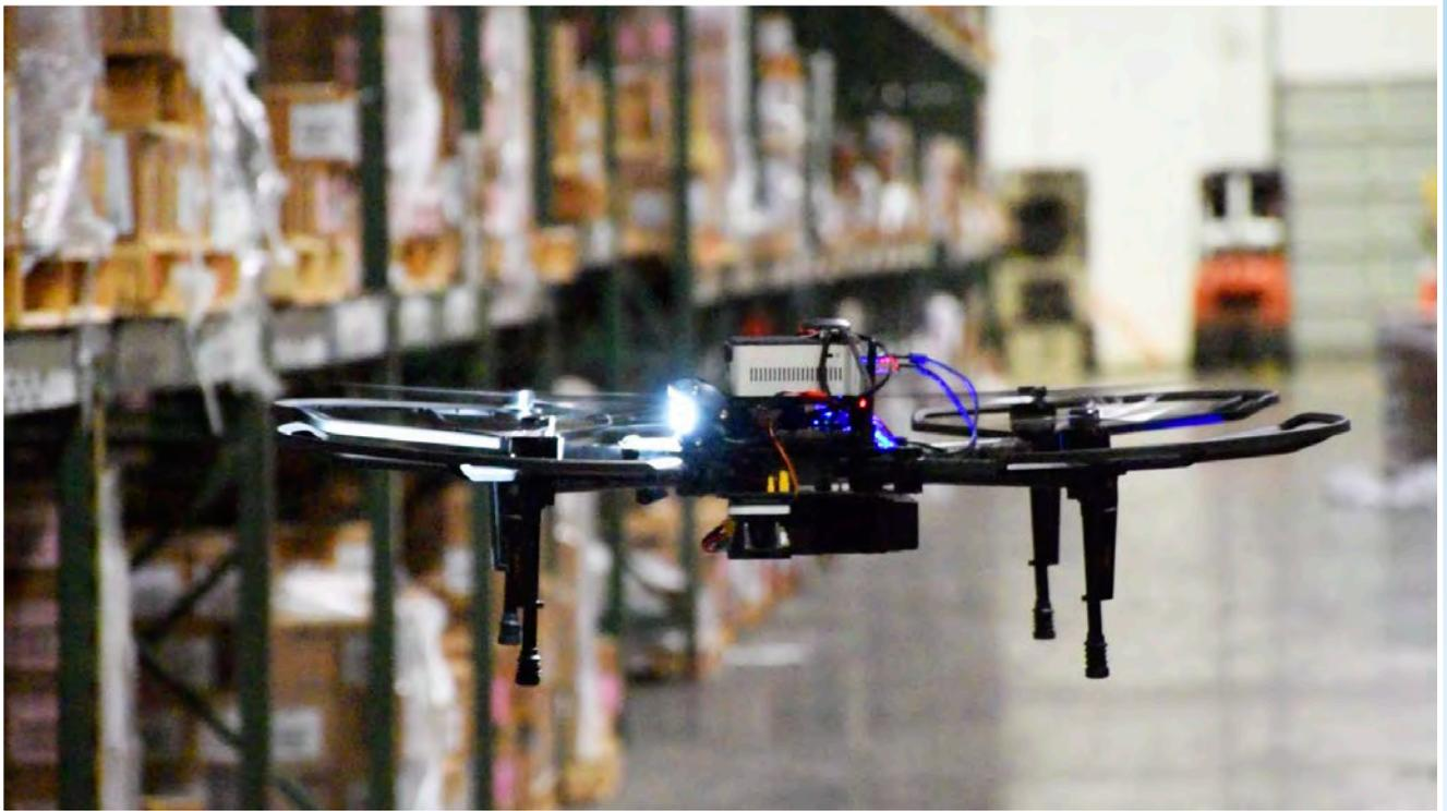
**PINC Solutions provides aerial robotic technology that can efficiently and effectively survey a wide area to autonomously locate and track inventory data and assets.**
