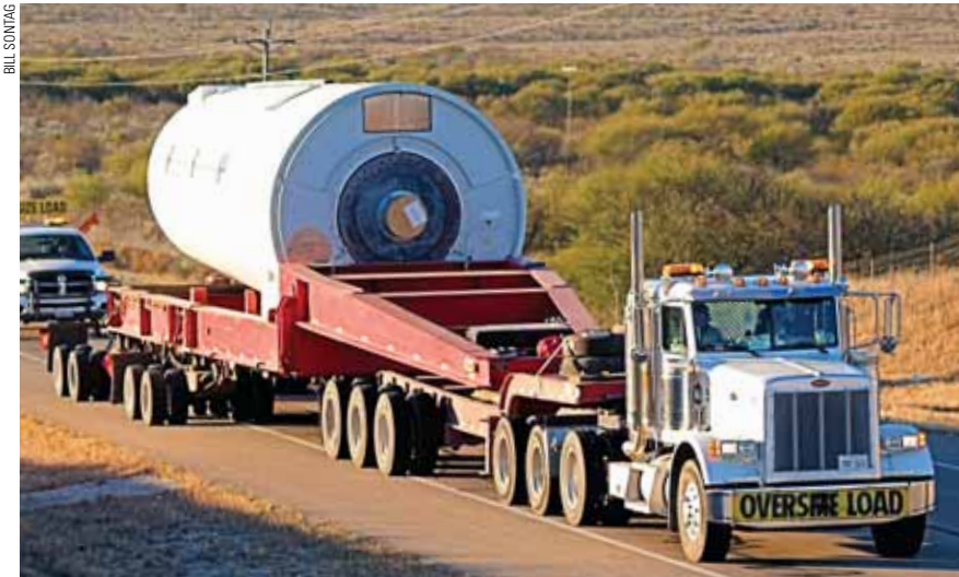
MASS(IVE) TRANSIT: Trucks transporting huge wind energy equipment are a common sight along the Corridor. It takes eight to 10 trucks just to haul the major equipment for one wind turbine, which might include a 250-foot tower and 120-foot blades.
