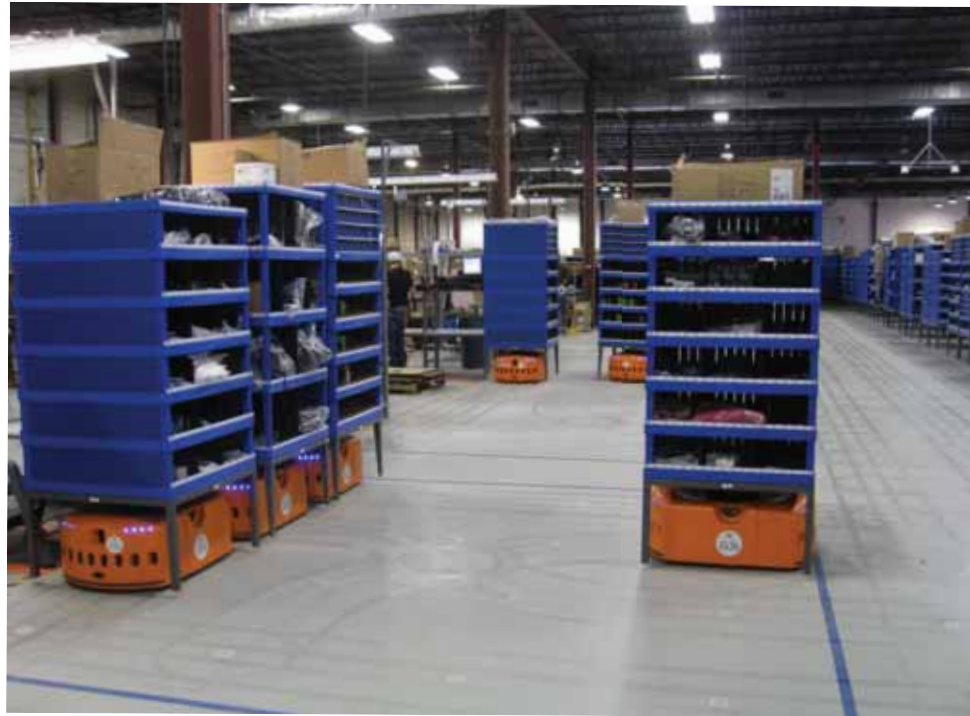
Quiet Logistics’ robotic warehouse fulfillment operation, powered by Kiva Systems, enables fully automated receiving, putaway, picking, packing, and shipping.
