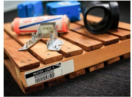
Pallets display the barcode label used to communicate with PathGuide’s WMS.
