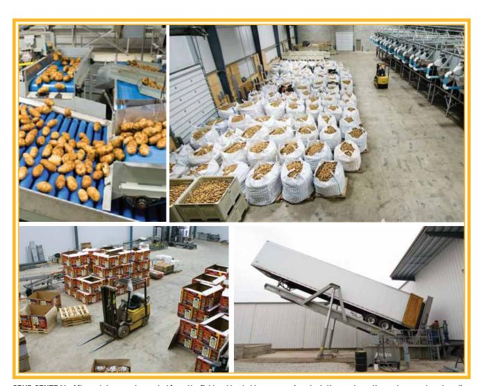
SPUD CENTRAL: After potatoes are harvested from the field and hauled to a processing plant, they undergo three-stage wash and grading processes to eliminate bacteria and sort for quality and size. Tubers are then packed to order or placed in temperature-controlled storage.
