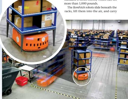
Mobile robotic drive units fetch inventory racks and zip them across Staples' distribution center to pick-and-pack stations. To avoid collisions, a computerized dispatcher sends each robot on a specific route across the facility's floor.
