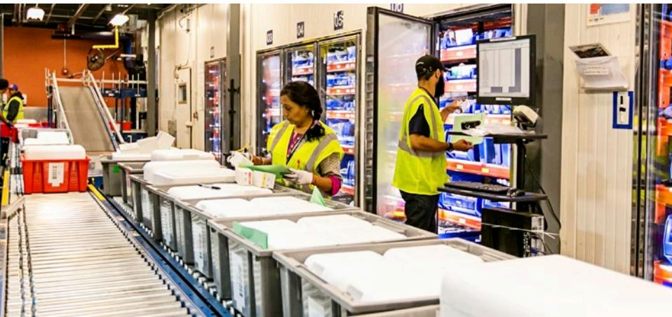
Pickers in Thermo Fisher Scientific's cold chain warehouse in Fredericksburg, Md., now fill orders in ambient temperature spaces. Deli-door style cases housing refrigerated products are on the first level; similar freezer cases are accessed via a second-level mezzanine.
