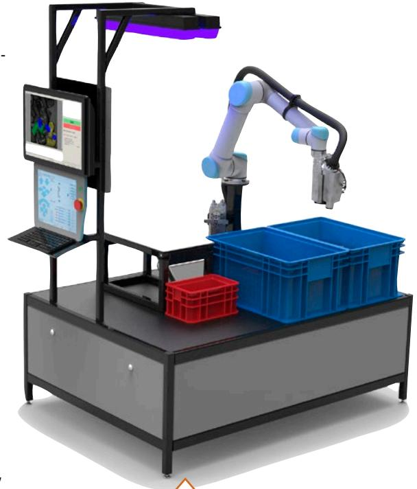
**Blue Ocean Robotics**, a provider of robots and automation solutions, released a standard solution for 3D bin picking of small industrial parts. The Mini-Picker bin picking solution is available with the Universal Robots UR5 collaborative robot. The system is designed for machine loading of small parts, and will soon be available with additional robot brands to cover a wider range of parts.
