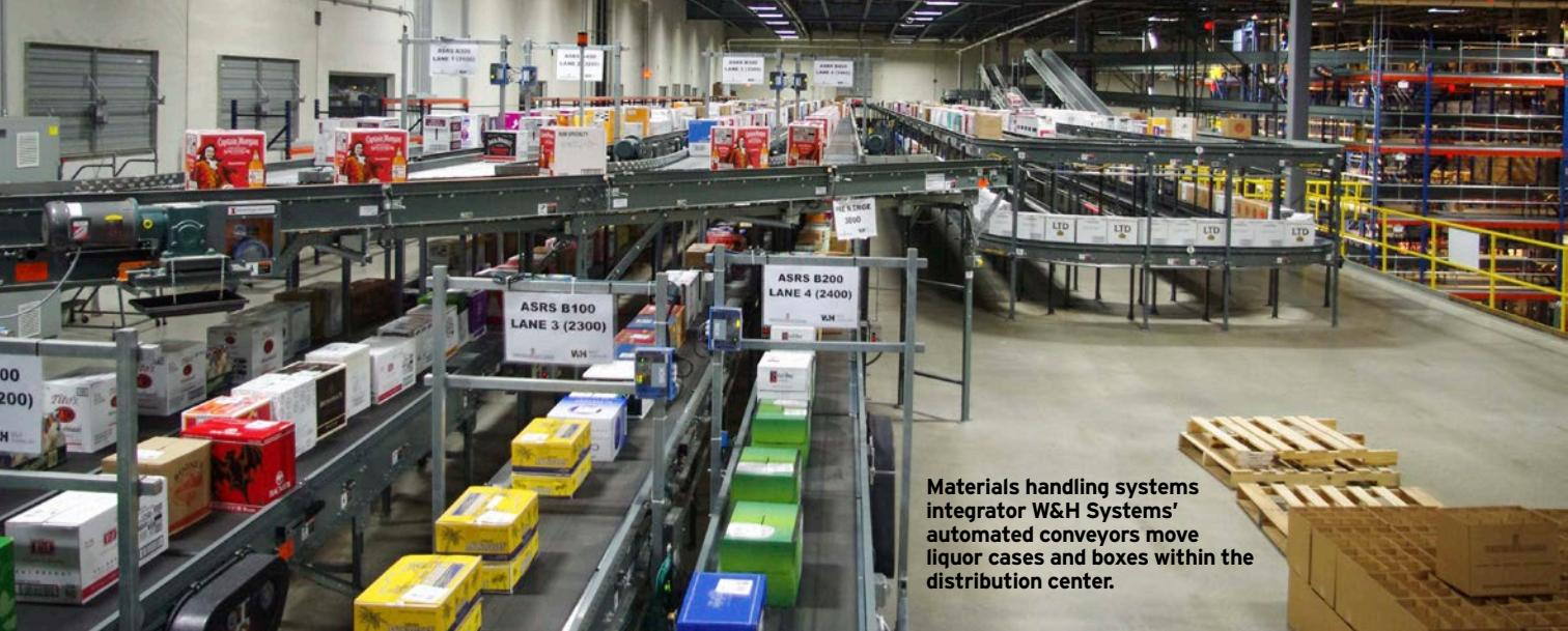
Materials handling systems integrator W&H Systems' automated conveyors move liquor cases and boxes within the distribution center.
