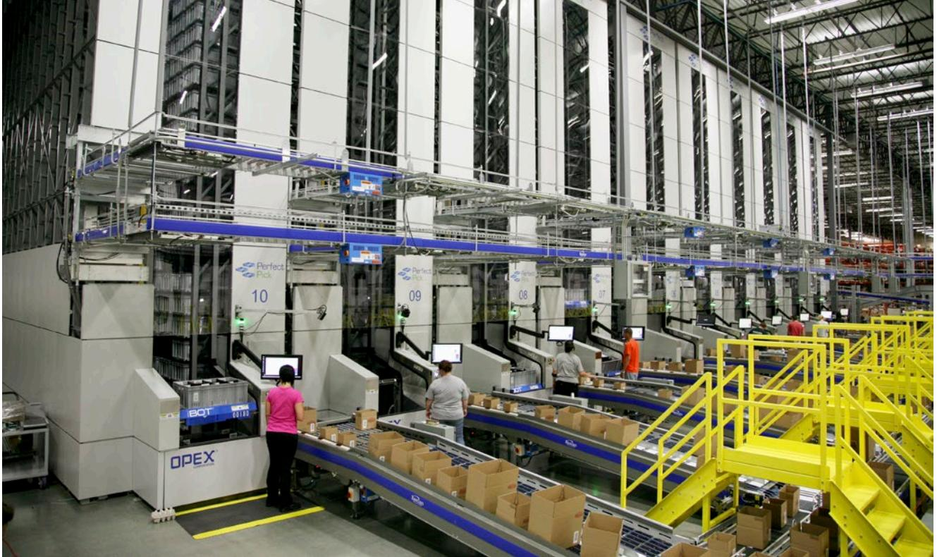
**In goods-to-person order fulfillment, product moves directly to the operator, who can then pick what is needed to fulfill orders. This system increases the efficiency and accuracy of the picking process.**
