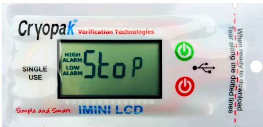
Cold chain solutions provider **Cryopak Verification Technologies** introduced its new iMINI LCD single-use temperature monitor to help shippers meet increasingly stringent regulations for temperature-sensitive shipments in the pharmaceutical and food industries. The device comes pre-programmed with shipper-provided specifications to allow for temperature monitoring within a shipment.
