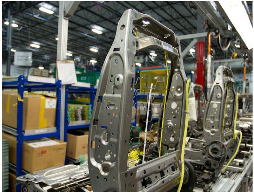
**Carton flow racks, such as those used in Johnson Controls’ 125,000-square-foot plant in Suwanee, Ga. - where seats, door panels, and other interior parts are assembled for the Kia Sorento - help create flexible, modular, and portable storage.**
