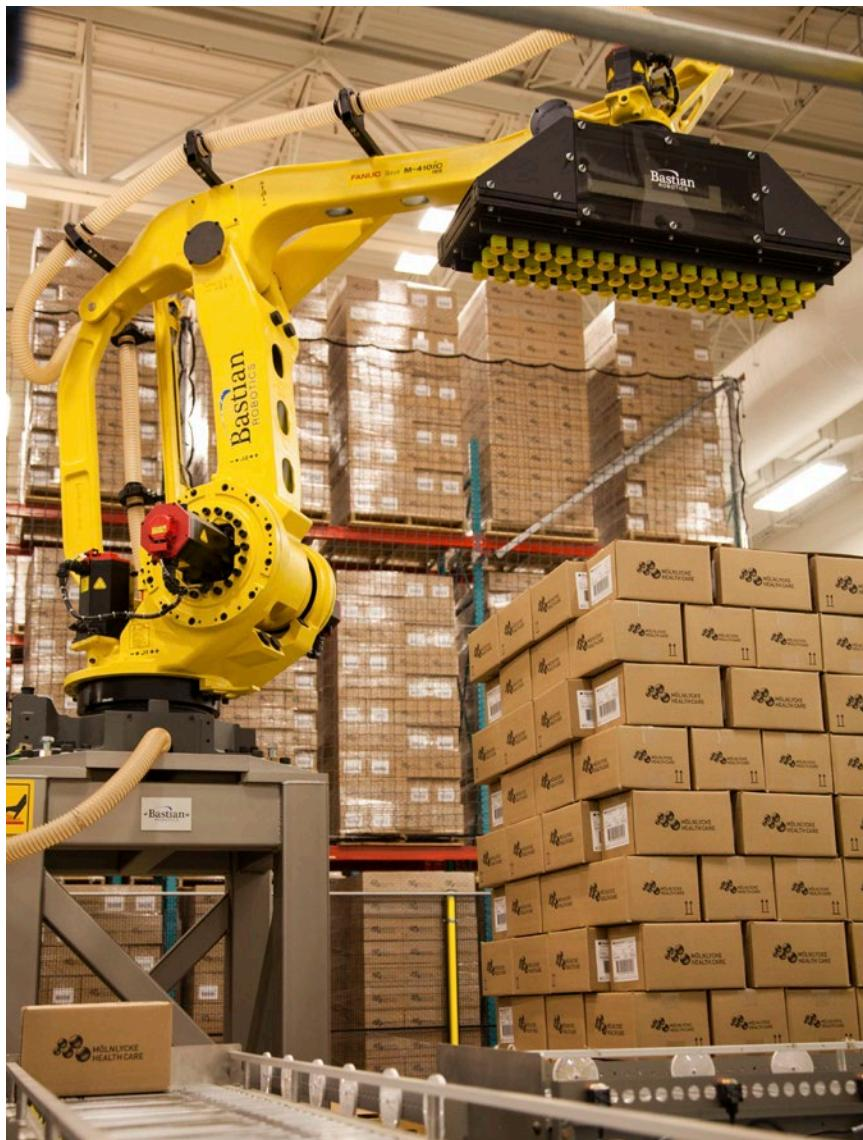
**Bastian's palletizing robots can handle pallets, slip sheets, and tier sheets for completely automatic pallet building and depalletizing operations.**
