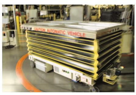
Magnetic tape placed on the warehouse floor directs automated guided vehicles to storage zones and workstations throughout the facility.
