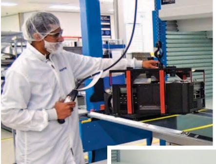
When a projector is ready for picking, the operator uses handheld controls to position the hoist near the desired projector, hooks the hoist onto the projector, lifts it into the air, and lowers it onto the cart.
