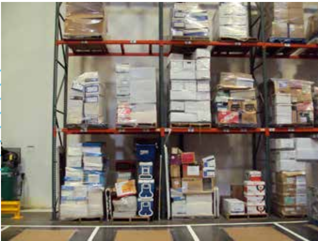
For one company, a disorganized rack system (left) wasted worker time and effort. After APL Logistics implemented the 5S Lean technique, however, workers can easily locate equipment and supplies (right).
