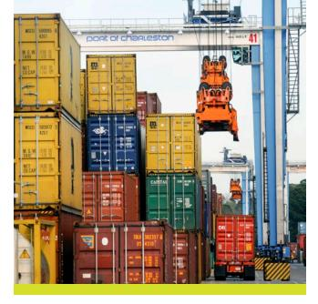
To reduce emissions, the Port of Charleston invested in fully electrified ship-to-shore and rubber-tired gantry cranes.
