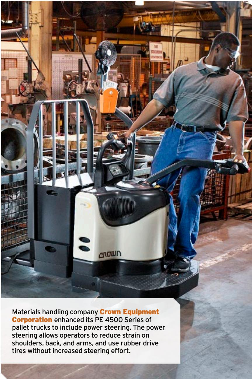
Materials handling company **Crown Equipment Corporation** enhanced its PE 4500 Series of pallet trucks to include power steering. The power steering allows operators to reduce strain on shoulders, back, and arms, and use rubber drive tires without increased steering effort.
