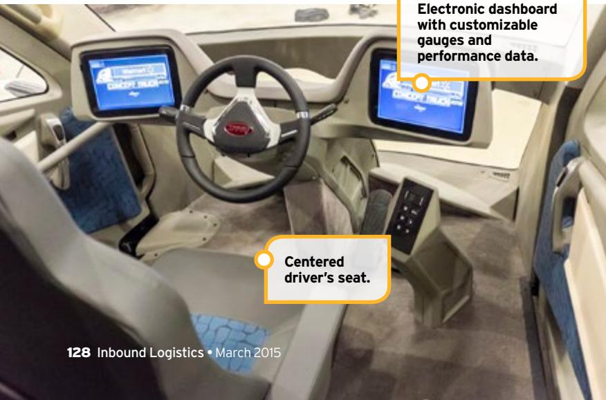
Electronic dashboard with customizable gauges and performance data.
