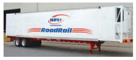
NFI RoadRail's refrigerated intermodal container is designed for double stacking on a railcar and triple stacking at the terminal.
