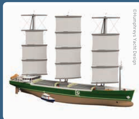
Rolls-Royce is developing a 4,500-ton ship primarily powered by a 180-foot sail, with bio-methane engines providing additional power.
