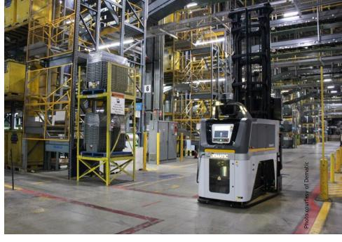
Automated guided vehicles (AGVs) follow markers or wiring on the warehouse floor and use lasers, voice activation, and magnets for navigation.
