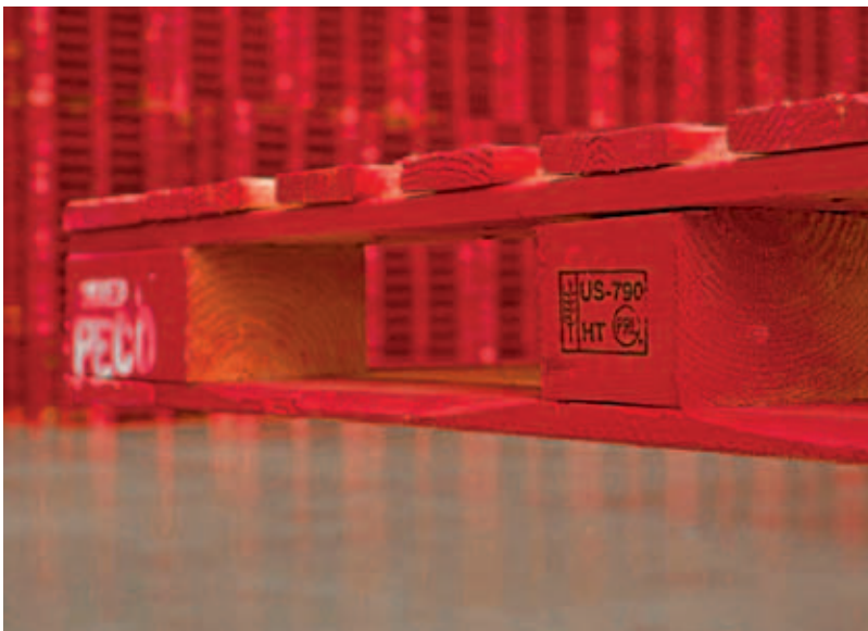
Four-way block pallets, which most pallet pooling companies use, are often made from a harder wood than conventional stringer pallets.
