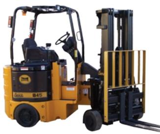
in highway trailers or travel through low doorways. Electric capacities range from 3,000 pounds to 4,500 pounds. The Bendi comes standard with an 11.8-inch stroke side shifter and can also be equipped with a variety of hydraulic attachments, such as paper roll clamps, drum clamp, and a carton clamp to further enhance versatility.
