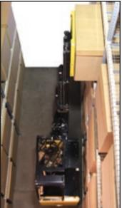
up to 33 feet. Its high productivity stems from a powerful combination of energy efficiency, ergonomic design, excellent load and fork visibility, and smooth lift hydraulics. Three standard driving programs are present to suit differing conditions and operator skills. Generous padding protects and supports the operator's legs and back during turns and braking, and the platform is low for easy mount and dismount.
