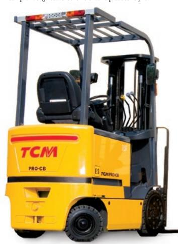
emissions, while running cooler due to an improved engine compartment airflow. The automatic transmission has cast iron cases; bigger shafts, gears, and torque converters; and clutch packs for reliability and quiet operation.
