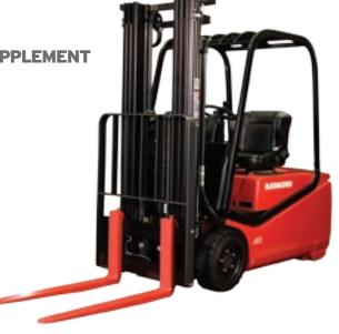
to shorter cycle time from dock to stock. Users also save money with longer brake life; oil cooled, these brakes last up to twice as long as dry friction brakes. A unique open view mast offers exceptional visibility and multiple height/stage options.
