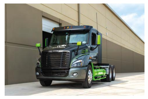
> Hyliion launched a fully electric, long-haul powertrain: the Hypertruck Electric Range Extender (ERX), which leverages an existing fueling infrastructure to offer fleets net-negative GHG emissions and low operating cost. With an electric drivetrain and a natural gas-powered onboard generator to recharge the battery, the Hypertruck ERX provides more than 1,000 miles of range.
