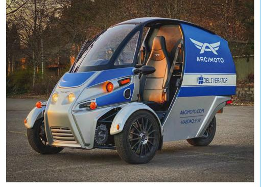
> The Deliverator, a three-wheel electric vehicle, is now available for rent in Los Angeles through the HyreCar platform, a carsharing marketplace. Vehicle maker **Arcimoto** and **HyreCar** launched the rental program to provide an efficient last-mile option. Arcimoto's vehicle has a 100-city-mile range, a 500-pound carrying capacity, and 20+ cubic feet of cargo space.
