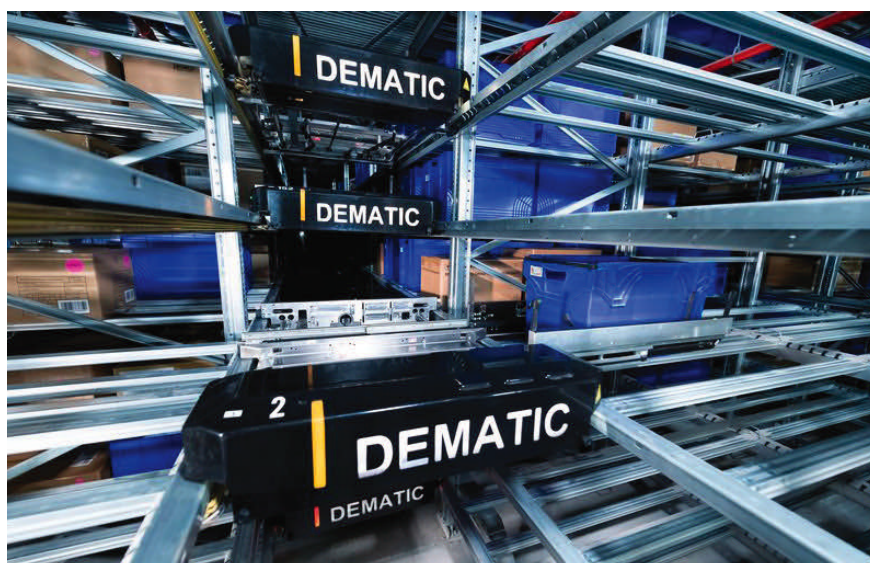
The Dematic Multishuttle stores, buffers, and sequences products between bulk stock and other functions such as picking and order assembly. These types of systems can increase speed, storage density, accuracy, and throughput in warehouses and distribution centers.
