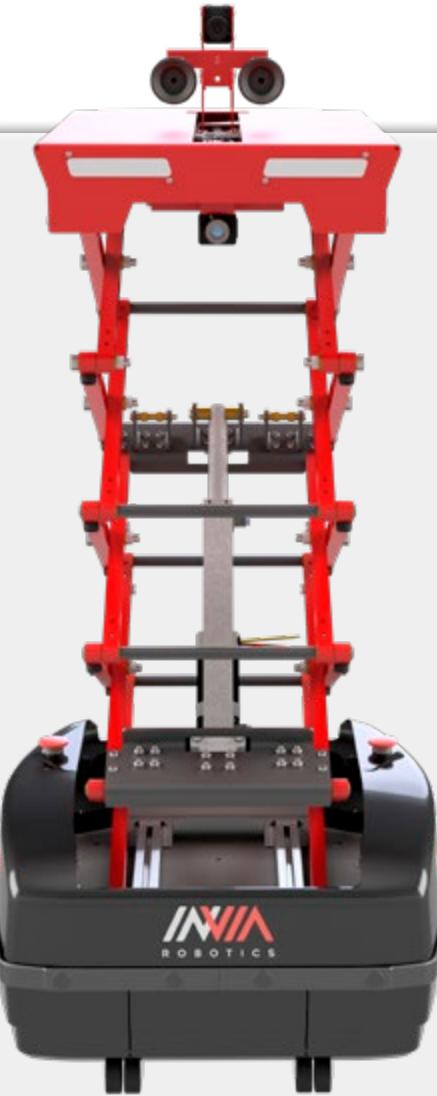
**inVia Picker:** Picking items as small as a pack of gum or as bulky as a case of soda, this robot provides a solution for e-commerce fulfillment centers through a Robots-as-a-Service platform. Pickers operate as an automated storage and retrieval solution, picking totes, bins, and boxes weighing less than 40 pounds from warehouse shelves. The robots can run on their own or work collaboratively with human operators.
