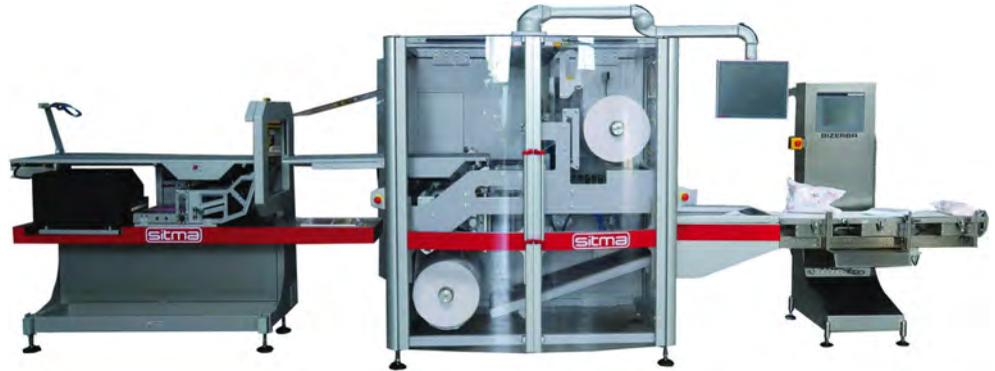
> Designed for e-commerce, **Sitma Machinery's** e-Wrap 2.0 can assemble packages and envelopes of varying sizes with different types of wrapping materials, including bio film and paper. The packaging machine can integrate a feeding system that prints and applies paper inserts, such as invoices, return notes, and other documents, to the packaging without glue.
