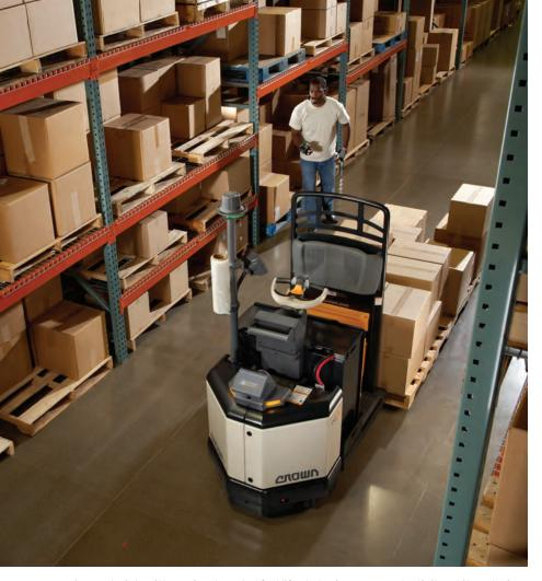
Moving materials with semi-automated forklifts helps improve productivity while reducing operator fatigue. Crown Equipment's QuickPick remote order picking system allows the operator to move the vehicle forward a pre-determined distance without getting back on the forklift.
