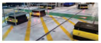
Auto guided vehicle company **Kivnon** installed a warehouse management platform for **Faurecia**, an automotive technology company, in Vitoria-Gasteiz, Spain. The system includes an end-of-line buffer, sequence, and warehouse as part of its car seat provision system.
