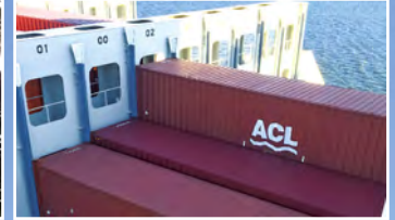
3,807 TEUs Container Capacity ACL's cell guide system safeguards containers and reefers on and below deck.
