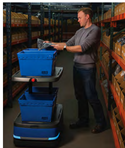
“Chuck,” an automated guided vehicle from 6 River Systems, navigates warehouse floors alongside staff to boost picking efficiencies.
