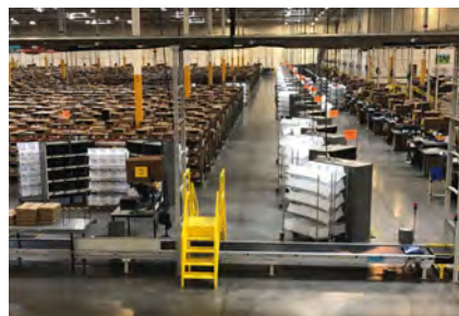
E-commerce fulfillment centers often feature lower-level picking and more conveyor belts than traditional warehouses.
