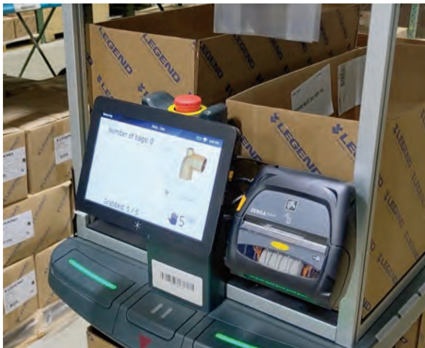
6 River Systems' collaborative Chuck robots display product photos on a monitor to make it easier for Legend Valve's warehouse associates to identify the products they pick. As a result, the plumbing wholesaler has increased order fulfillment accuracy.
