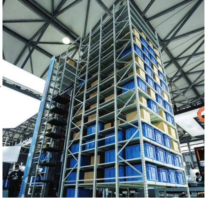
> The new RoboShuttle from **Geek+** allows businesses to make full use of vertical warehouse space and store, retrieve, and organize boxes carrying small to mid-sized items. RoboShuttle can identify and place boxes of popular SKUs on the lowest shelf to speed up the picking process, handling up to 500 boxes/hour/station.
