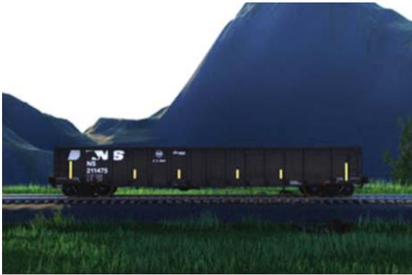
▲ **U.S. Steel, Norfolk Southern, and The Greenbrier Companies** are creating a sustainable steel gondola railcar, which transports loose bulk material. Using a formula for lighter-weight steel developed by U.S. Steel, each gondola's weight decreases by up to 15,000 pounds. Norfolk Southern will acquire 800 of the Greenbrier-engineered gondolas.
