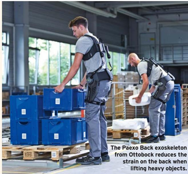
**The Paexo Back exoskeleton from Ottobock reduces the strain on the back when lifting heavy objects.**
