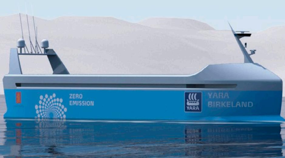
The *Yara Birkeland* will be the world's first fully electric and autonomous container ship, with zero emissions. Unmanned voyages are planned for 2020.
