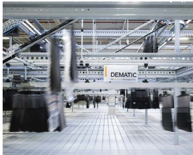
The Dematic Pouch System uses pouches and hooks, each carrying a single item, suspended from rolling adapters that move along ceiling-suspended rails. The system can store, transport, sort, and sequence items in support of e-commerce and omnichannel order fulfillment.
