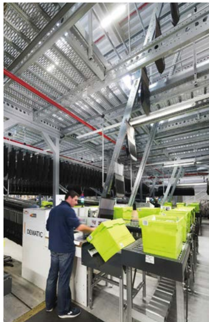
The Dematic Pouch System uses pouches and hooks, each carrying a single item, suspended from rolling adapters that move along ceiling-suspended rails. The system can store, transport, sort, and sequence items in support of e-commerce and omnichannel order fulfillment.
