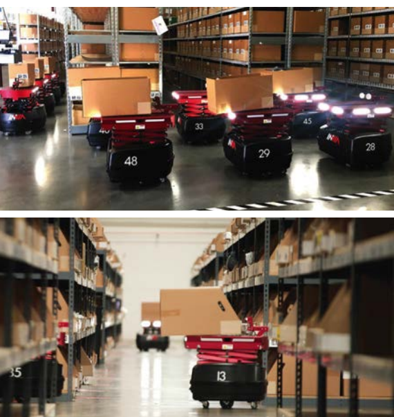
inVia robots work autonomously to retrieve and move goods in the warehouse, eliminating the need for workers to walk through aisles. They also calculate the most efficient path to follow.
