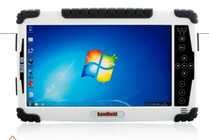
The Algiz 10X rugged tablet from **Handheld US** provides mobile computing capabilities for any environment. The tablet has built-in GPS, a variety of Internet connection options, and a 5.0 megapixel camera. It weighs only 2.9 pounds, allowing for use in many transportation, yard, and warehouse applications.
