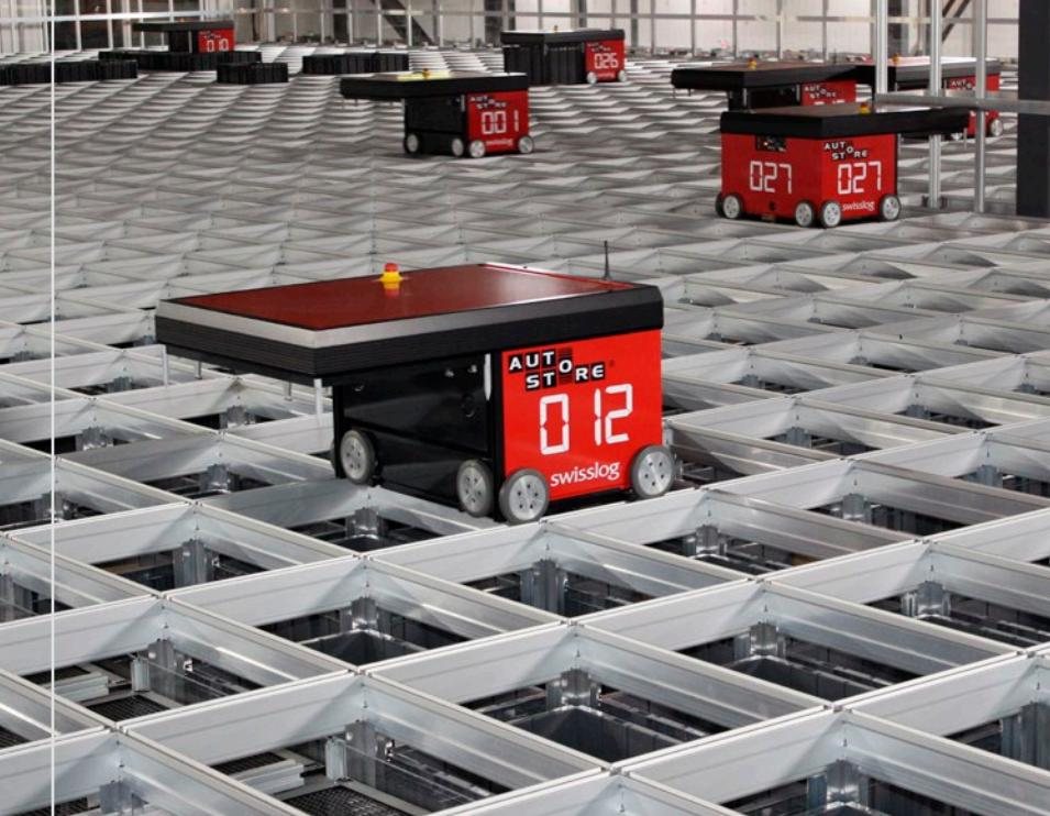
**Robots with transport and lifting functionality operate Swisslog's AutoStore system. Equipped with a lift, robots retrieve the required bins from the AutoStore grid and present them at integrated picking stations, led by a controls and location management system.**
