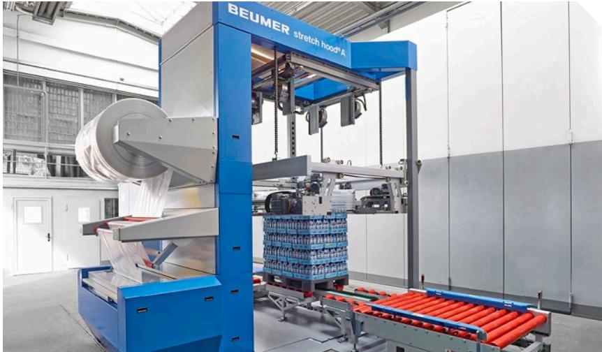
Conveying systems maker **BEUMER Group** unveiled its new stretch hood high-capacity system. The machine series offers higher throughput, and gentle transport of the film in the system. It also requires 40-percent less floor space than older systems. In addition, its opening hood lets workers in retail stores and logistics centers quickly remove the film when unpacking or repacking the goods, without using any cutting tools.
