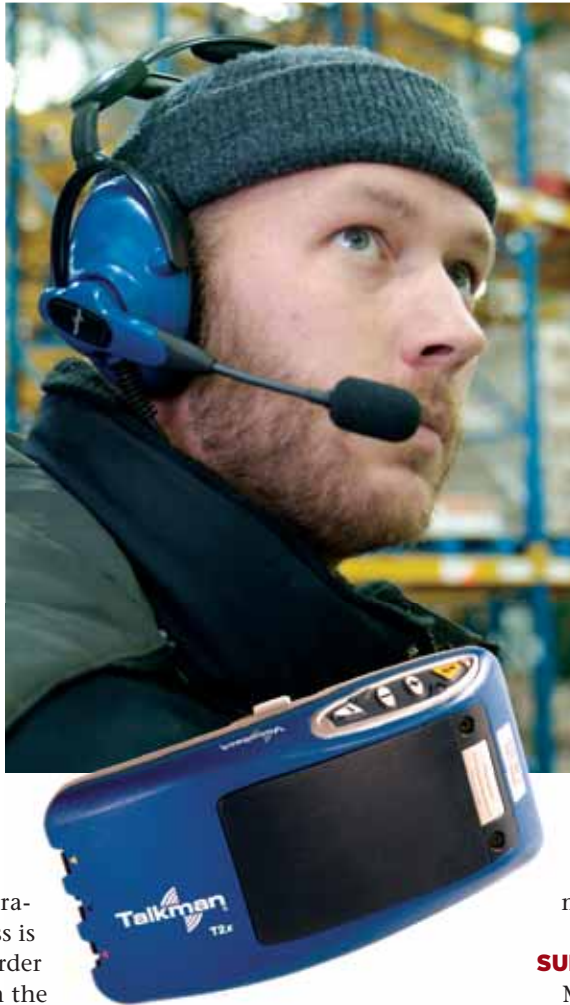
Vocollect's Talkman wireless computers (below) attach to a worker's belt and plug into headsets (above), which allow Dreyer's Edy's workers to hear automated work instructions in the refrigerated warehouse.
