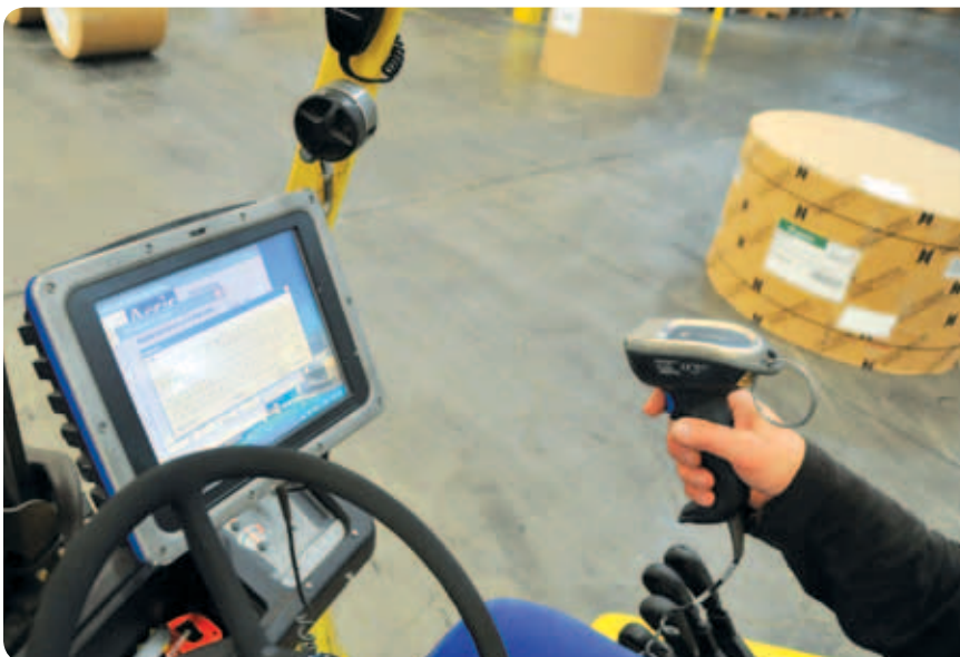
Truck-mounted computers (above) collect and report inventory data for products received, stored, and shipped from Roosevelt Paper’s warehouse, while wireless printers (top) print customized barcode labels on demand.
