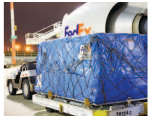
To protect temperature-sensitive pharma shipments, FedEx uses tools such as thermal blankets (above) and SenseAware devices, which contain sensors that monitor temperature, light exposure, humidity, and other factors that might affect drugs in transit.
