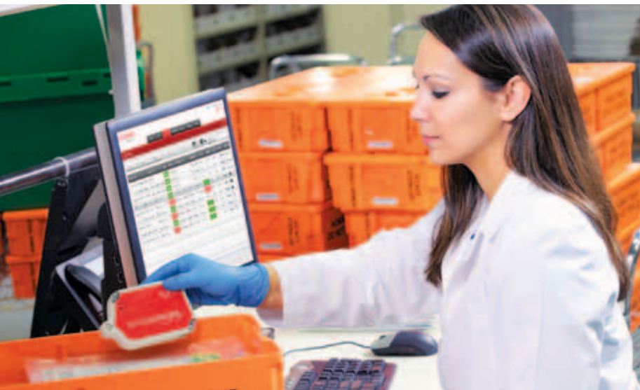
To protect temperature-sensitive pharma shipments, FedEx uses tools such as thermal blankets (above) and SenseAware devices, which contain sensors that monitor temperature, light exposure, humidity, and other factors that might affect drugs in transit.
