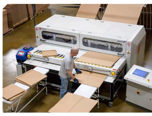
Solutions such as Box On Demand's system quickly and cost-effectively produce custom corrugated packaging, allowing shippers to keep packaging costs consistent across any configuration, quantity, or design.
