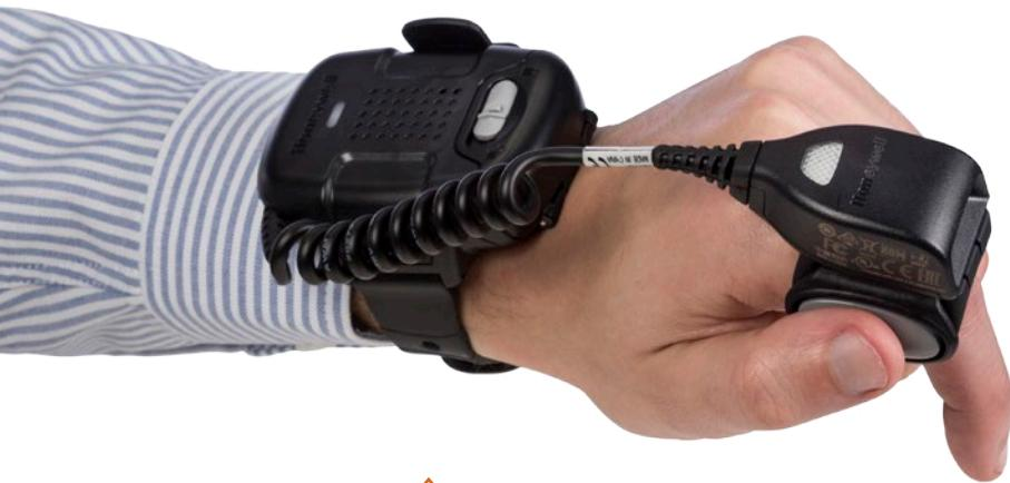
**Honeywell** released its 8670 Wireless Ring Scanner with Bluetooth technology, a compact, lightweight scanner that fits comfortably on a finger to allow workers to keep both hands free when completing their tasks. The new ring scanner is designed for use across all areas of a distribution center. It uses Bluetooth technology to connect to a range of computing devices such as PCs, laptops, tablets, vehicle-mounted computers, rugged mobile computers, and smartphones.
