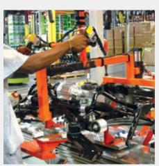
The Lordstown plant produces about 1,000 Cruze models daily. Split-second timing is crucial on the drive train assembly line (above), where parts arrive at the exact moment they're needed.
