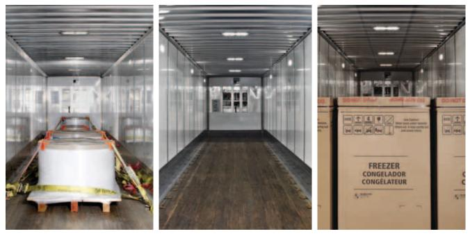
The X-duty trailer carries heavy-duty raw steel coils to the Electrolux manufacturing plant; it is then unloaded, and refilled with finished goods for outbound haul.
