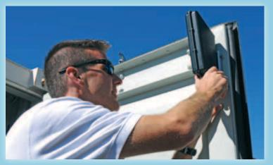
Georgia Tech Research Institute developed the Container Security Device to detect unauthorized opening or removal of marine container doors. The device was designed to withstand harsh shipping environments.
