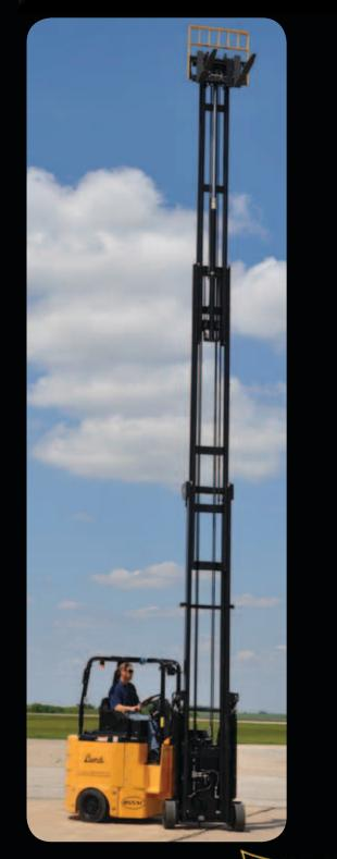
With lift heights to 473"(12M) and a stacking aisle of 84" (2.13M) the New Bendi Model B55ACHL provides a superior Narrow Aisle solution for maximum utilization of cubic storage space. The B55AC-HL has a basic capacity of 2.25 Tons and can lift 1 Ton at maximum lift height.
