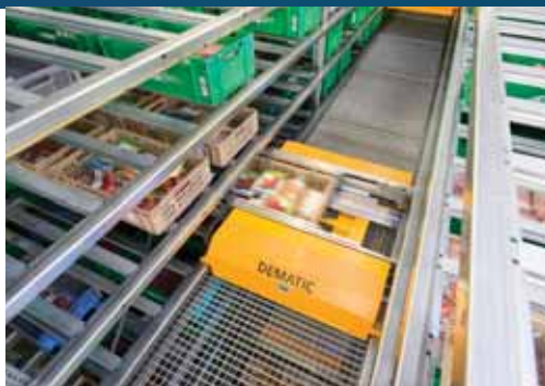
Dematic Multishuttle with DC electrical system is low energy user
