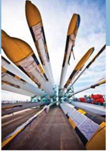
In addition to being highly engineered and sensitive, wind turbine blades are matched and balanced, and must be delivered to the iob site in sets.
