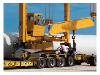
Careful handling, detailed planning, and specialized loading and hauling equipment are needed to move oversize and overweight wind power components from port to site or plant to site. (Photo courtesy of Landstar System)
