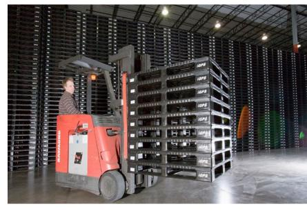
iGPS offers plastic pallets that lack the protruding nails and splinters that sometimes injure workers and damage products and equipment.
