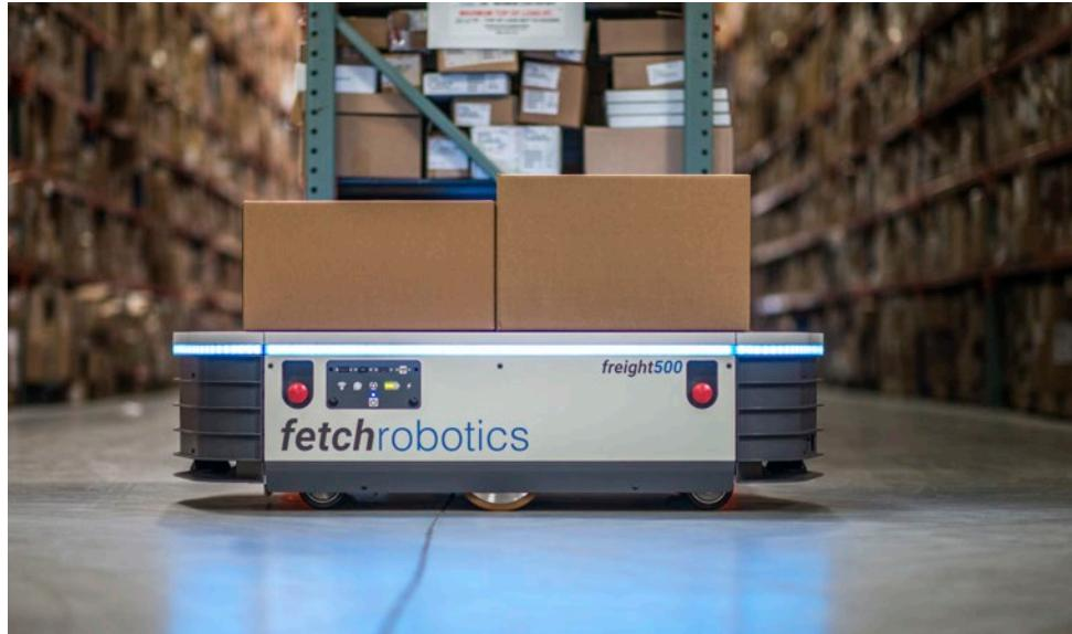
**Fetch Robotics** introduced two autonomous mobile robots to its fleet: Freight500 and Freight1500. Both new robots automate the delivery of bulky and heavy loads. Freight500 can move substantial loads, yet still fits through doorways and areas that people commonly traverse. For even bigger hauls, Freight1500 can support up to 3,300 pounds. Freight1500 can move standard-sized pallets as well as much bulkier cargo.
