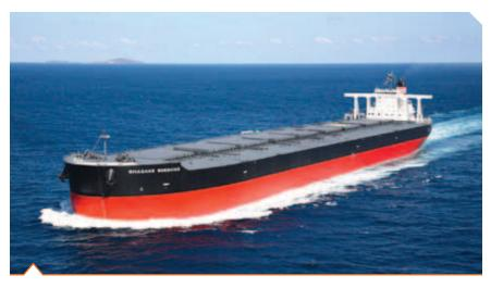
NYK Line added the 250,000-DWT class ore carrier Shagang Sunshine to its fleet. The vessel was built to carry the maximum loading capacity allowed at ports in western Australia, and will transport ore and coal from Australia to China.
