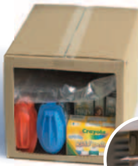
Step 2 Carton is Sealed and Bag is Inflated Automatically
