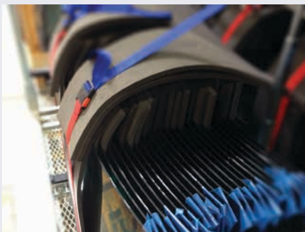
Auto glass manufacturer and distributor Safelite Group designed a collapsible steel pallet that allows it to move more windshields per pallet, while eliminating dunnage.
