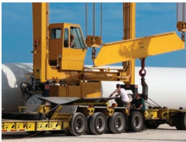
**Careful handling, detailed planning, and specialized loading and hauling equipment are needed to move oversize and overweight wind power components from port to site or plant to site. (Photo courtesy of Landstar System)**
