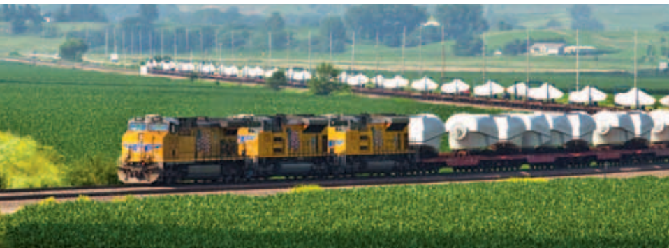
Transporting wind power components by rail allows shippers to circumvent some of the complications involved in moving the large equipment over the road.
