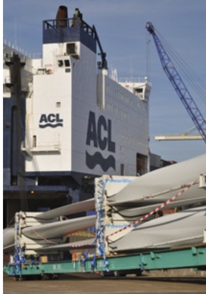
Garage decks on ACL's RoRo ships protect wind power equipment from the elements during transit.
